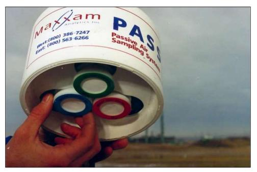
*Plate 1.* SO<sub>2</sub>, NO<sub>2</sub>, and O<sub>3</sub> sample filters attached to the rain shelter.
