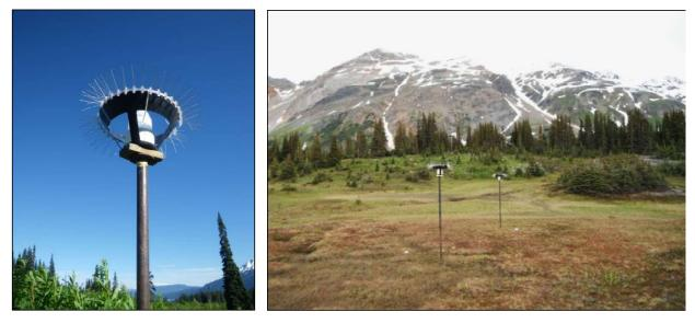
*Plate 1. Dustfall container inside wind shield housing.*
