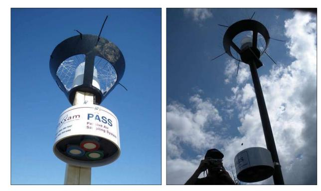
*Plate 2. Pass Filters in Rain shelter attached to wood dustfall stand.*
